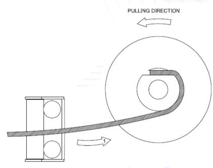
• If you mounted the Hydraulic winch using a bracket, the rope must be assembled as shown in the drawing.
