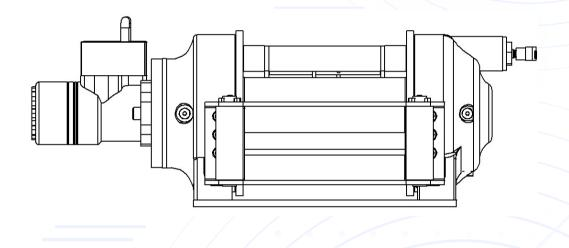
The assembly is made on a flat metal sheet. The thickness of the metal sheet on which the Hydraulic winch is planned to be assembled must be at least 15mm (For TORAco THW-22K, TORAco THW-26K, TORAco THW-33KSeries)
